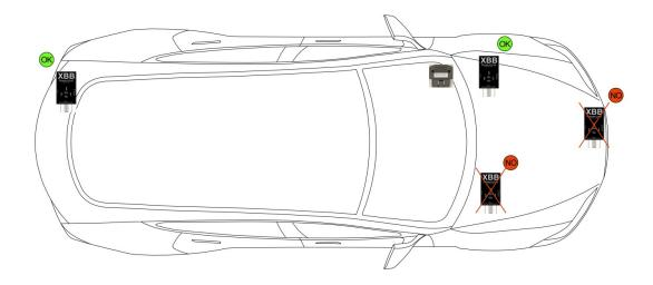
Keep the distance between the XBB Dongle<sup>®</sup> and XBB PowerUnit-6<sup>®</sup> as short as possible. In some rare conditions the vehicle and engine compartment will work as two different faraday's cage which may cause malfunction to the Bluetooth<sup>®</sup> connection.
